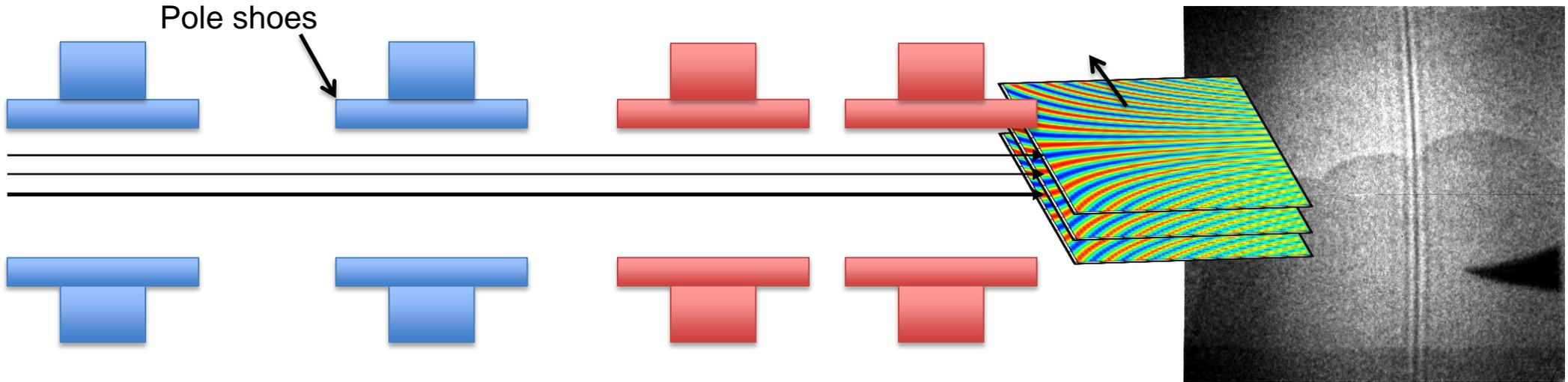
Schematic side view. Pole shoe distance: 60 mm, beam height 20 mm
